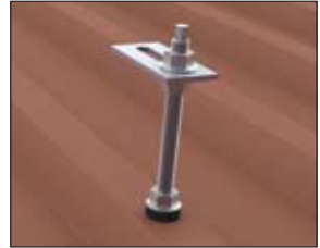
Position of the hanger bolt always on the wave crest not in the wave trough.
