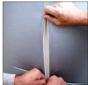
Watch out when closing the zipper (danger of tearing the insulation when not warm enough) Do not use a tong or any other tool.
