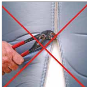
Watch out when closing the zipper (danger of tearing the insulation when not warm enough) Do not use a tong or any other tool.
