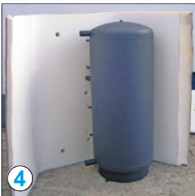
Only mount insulation when pre-heated! Pre-heat it for 24 hours to at least of 22 °C.
